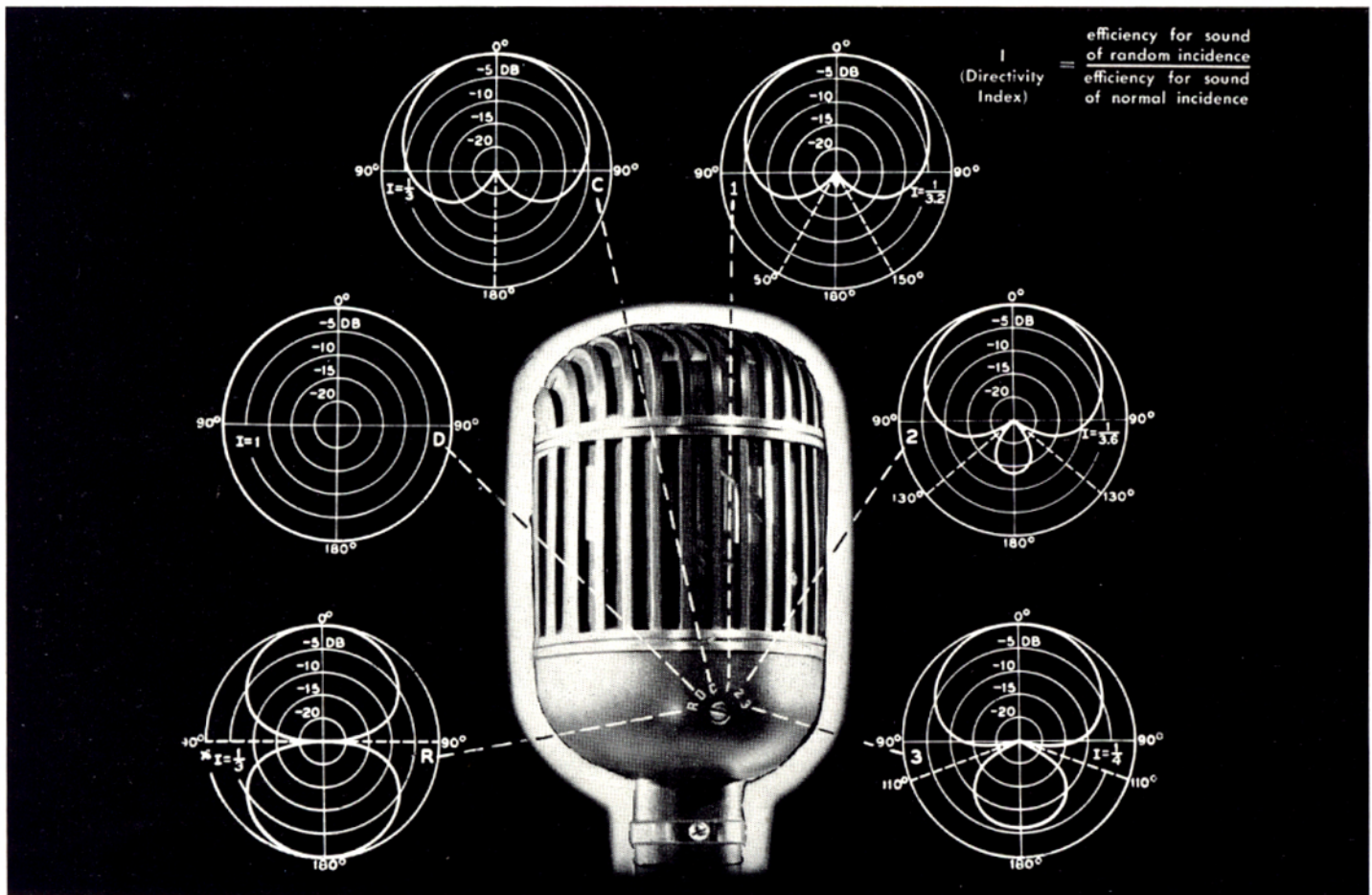
Figure 2 — Cardioid Microphone 639B showing 6 selectivity patterns.
