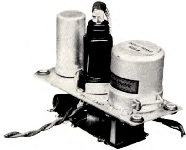
Figure 19 — 116B Pre-Amplifier used in 124F, 124G, and other amplifiers. Employs d-c bias gain control.
