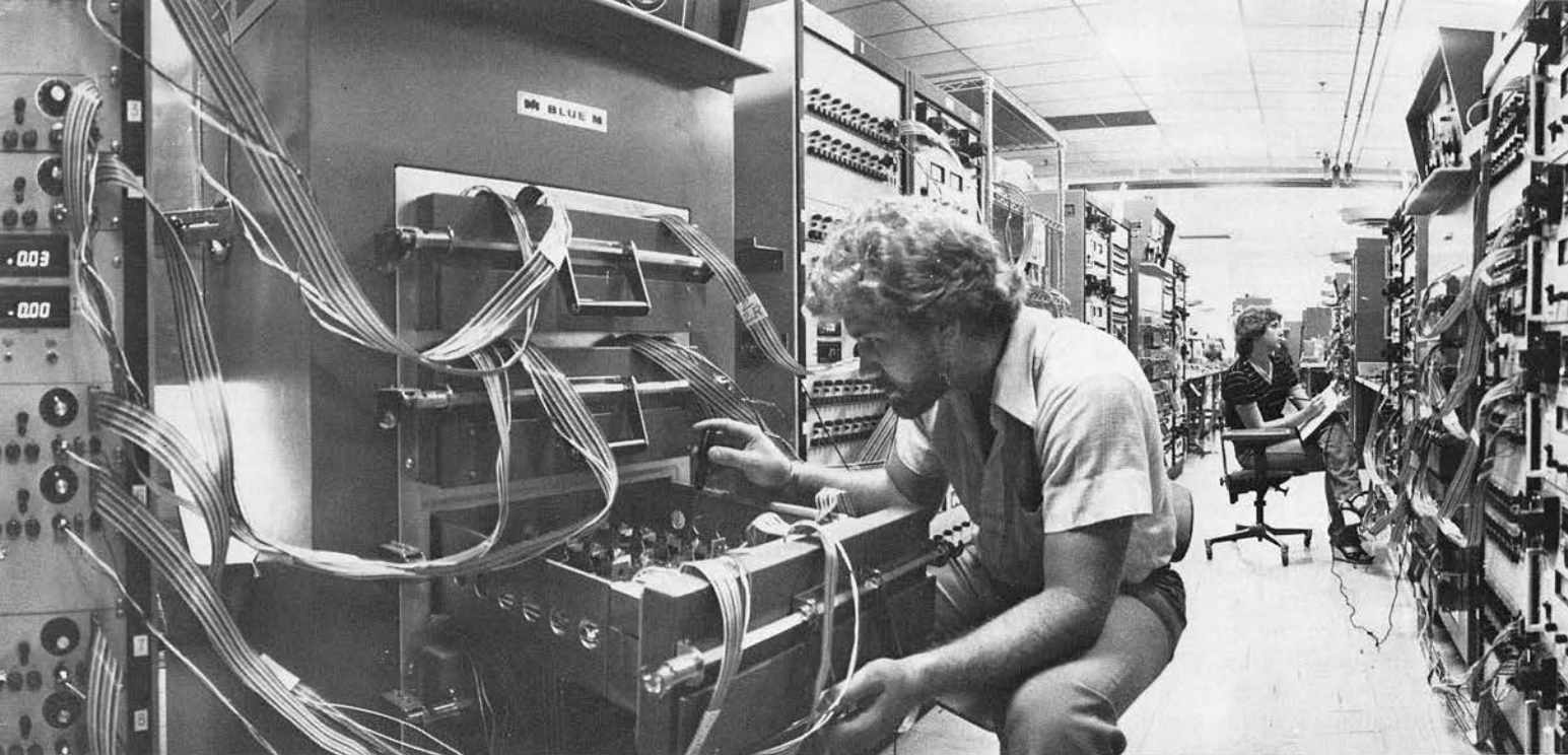
ABOVE—At Reading, John Sepko (foreground) checks a loose wire in a heat chamber where sample chips of gallium arsenide undergo extensive tests before the rest of a wafer is processed. In the rear, Linda Feick is taking readings.
