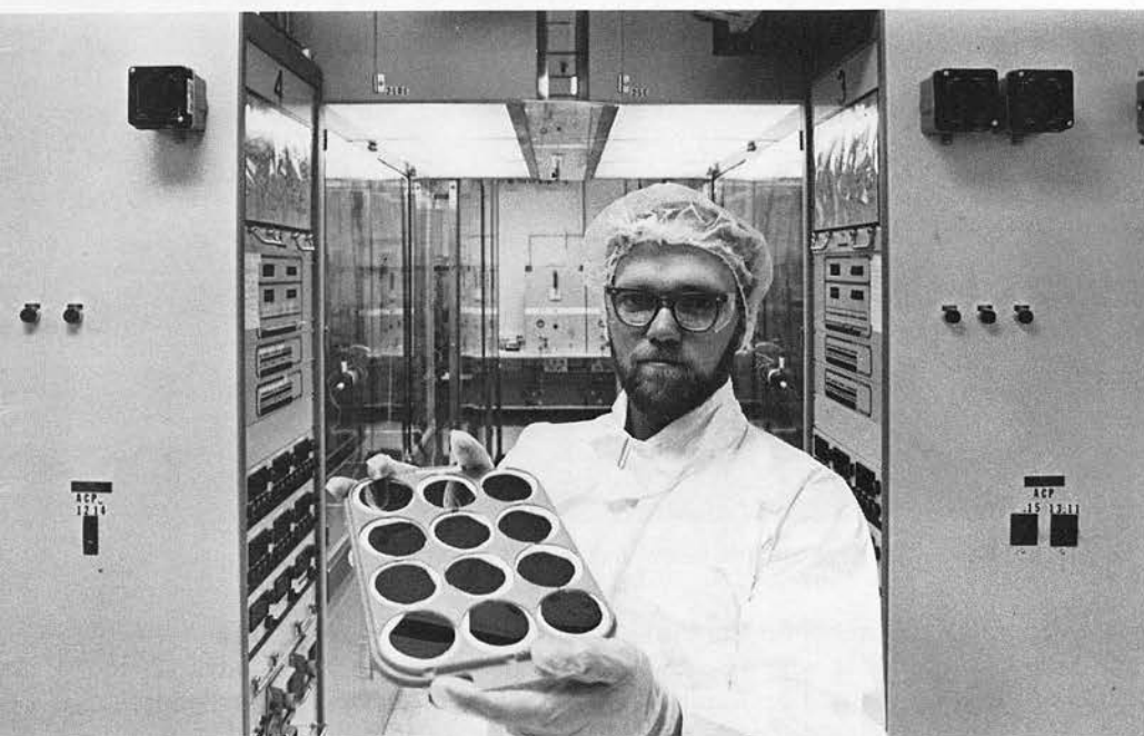
Surrounded by reactors in a newly completed clean-air building at Reading Works, Don Hartman shows a tray of substrates used for making GaAs Fets (gallium arsenide field effect transistors).
