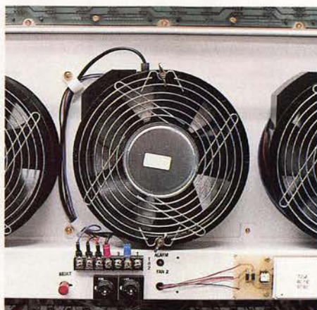
Built-in fans air cool circuit packs.
