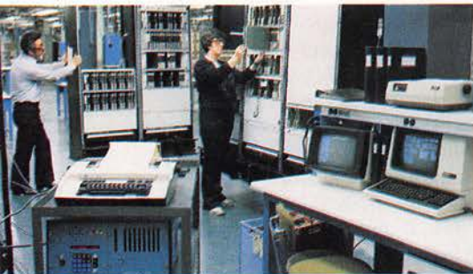
Mel Gering and Janet McReynolds test Interface Modules for the 5ESS switch.
