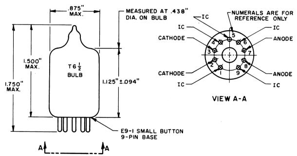
NOTE: PINS MARKED IC (INTERNAL CONNECTION) SHOULD NOT BE CONNECTED TO ANY PORTION OF AN EXTERNAL CIRCUIT. FAILURE TO OBSERVE THIS PRECAUTION MAY RESULT IN IMPROPER OPERATION OF THE TUBE.
