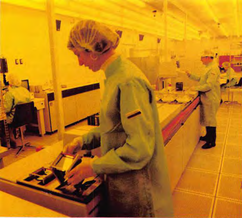
An automatic processing line for silicon wafers in the BIC clean room. Laurine Dietrich (foreground) loads machine while Jim Kamyniski adjusts controls. Picture was shot through yellow glass window.
