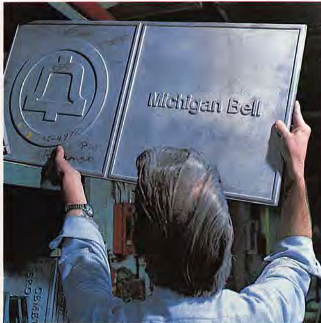
Standard patterns are re-usable. After twelve years of making Bell System signs and logos, almost every pattern is already on hand.
