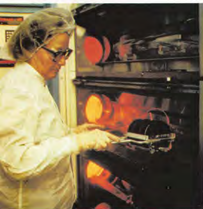
Norma Bloss prepares to load a tray of silicon wafers into a diffusion furnace. Microprocessors control and monitor the entire process.
