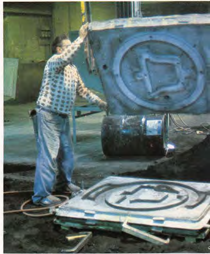
Above—The pattern vanishes under a finely-sifted layer of green sand. Once compacted, the sand holds the logo's shape tenaciously.
