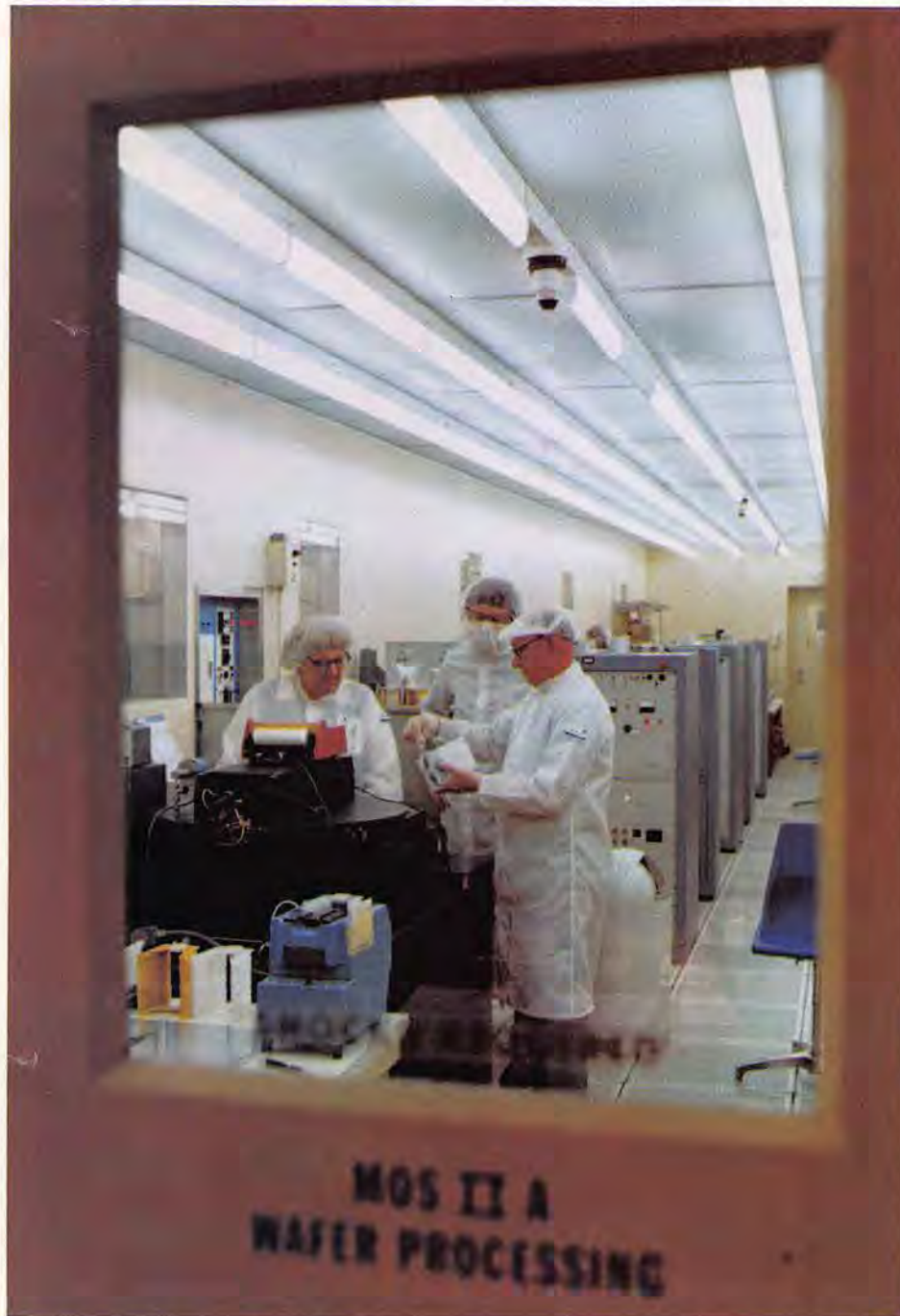
Checking a silicon wafer of VLSI chips are Theresa Neupauer, Tom Oswalt and Walter Held. The scene was photographed through window of the MOS clean room. Oswalt's beard is masked by snood to satisfy regulations.
