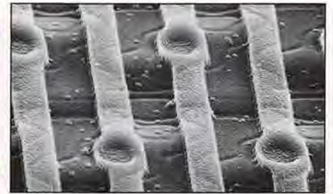
Microphotograph of metal contact strips on a 64K RAM. Each strip is much smaller than a human hair.
