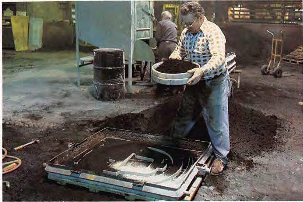
Above—The pattern vanishes under a finely-sifted layer of green sand. Once compacted, the sand holds the logo's shape tenaciously.
