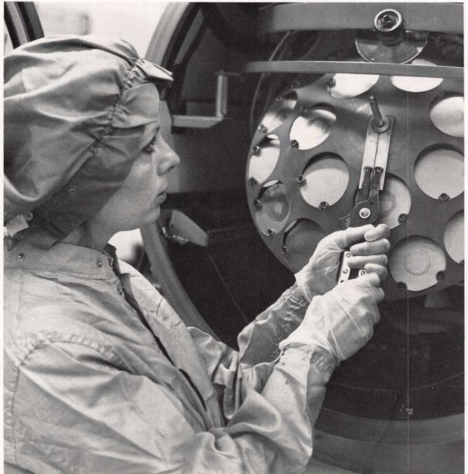
Evvi Ross of the Reading Works displays a "planet" of 21 gated diode wafers before loading into a machine that deposits a thin aluminum film on them.
