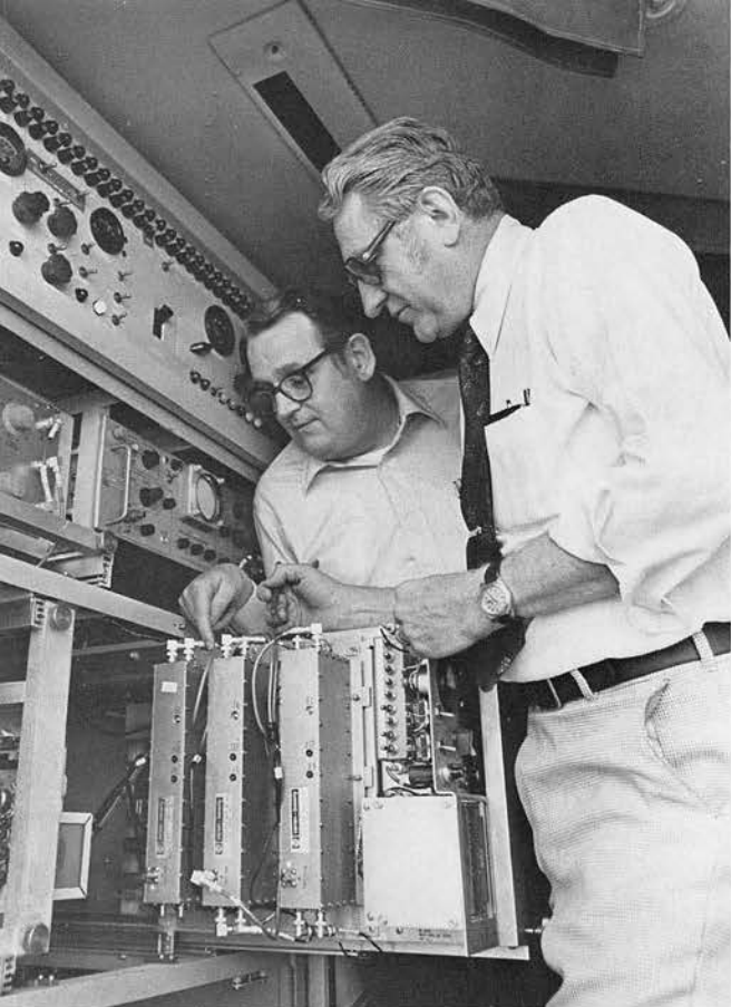
Left—In a Nike Hercules van returned for updating, Charley Pugh and engineer Len Dvoracek examine an IF amplifier. Above—Vernon Jones looks over a sonar data recorder, in for modification, that he built 20 years ago at the old Greensboro location.
