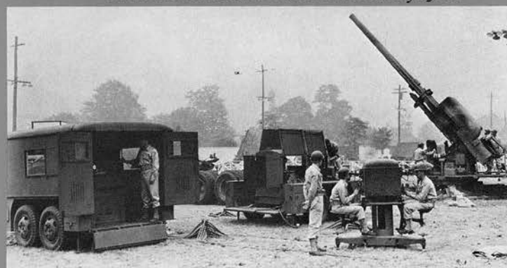
The Western Electric M-10 electrical gun director, which continuously and automatically set fuses on shells and aimed this 120 mm anti-aircraft gun.
