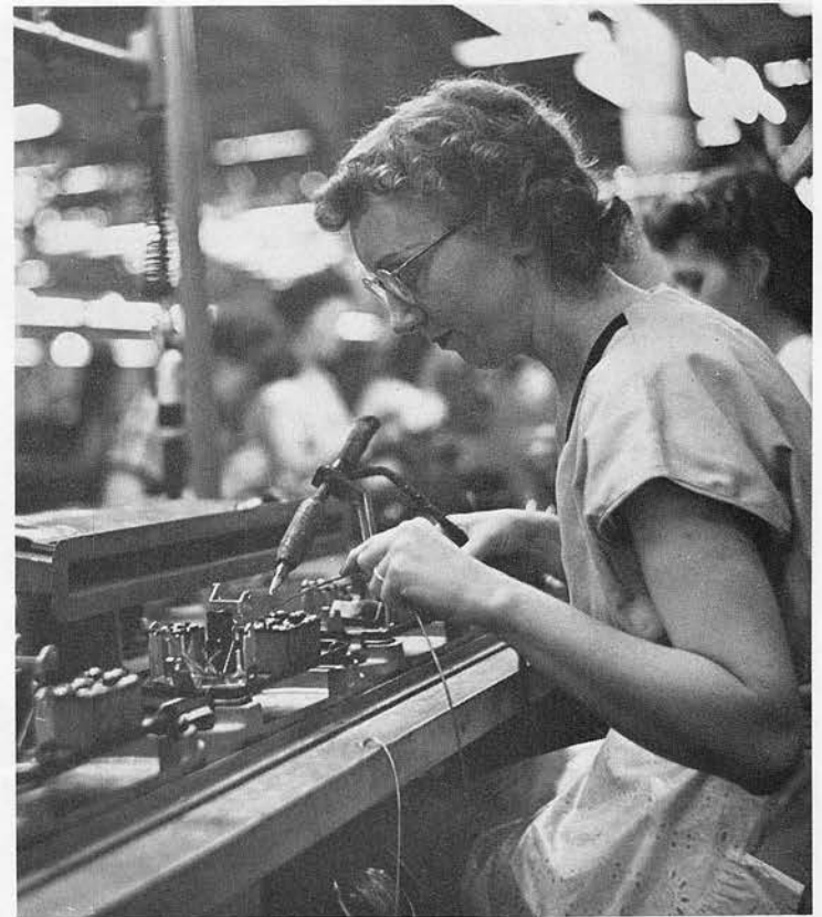
This one wasn't easy — at least not for your editors, who were off by more than a decade. The original caption said she's soldering terminals on the base of the new 500 set which should give you a hint. The place is the Indianapolis Works. The year? 1951.
