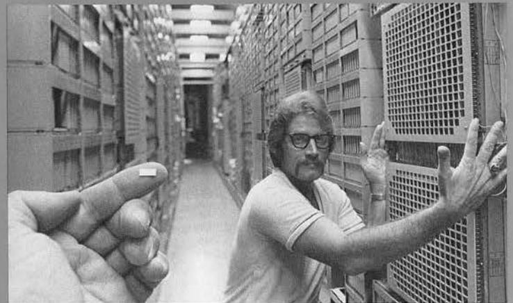
In this shot posed in a Long Lines office at the end of the decade, the pace of technological change is dramatically displayed. The tiny chip, from a 3B Processor, contains the equivalent memory of the large units indicated by the man's outstretched hands.
