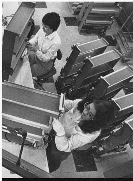
Assembling shelves for a SLC-96 unit are Kaye Griener and Mary Galloway at the North Carolina Works.
