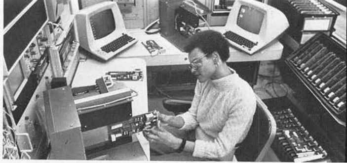
Cender Reed runs the final assembly tests of channel units for SLC-96.
