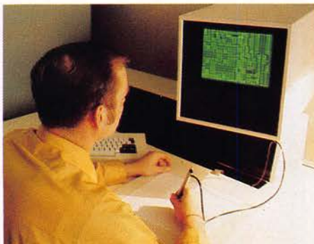
Computer aided design is used to lay out circuit boards.
