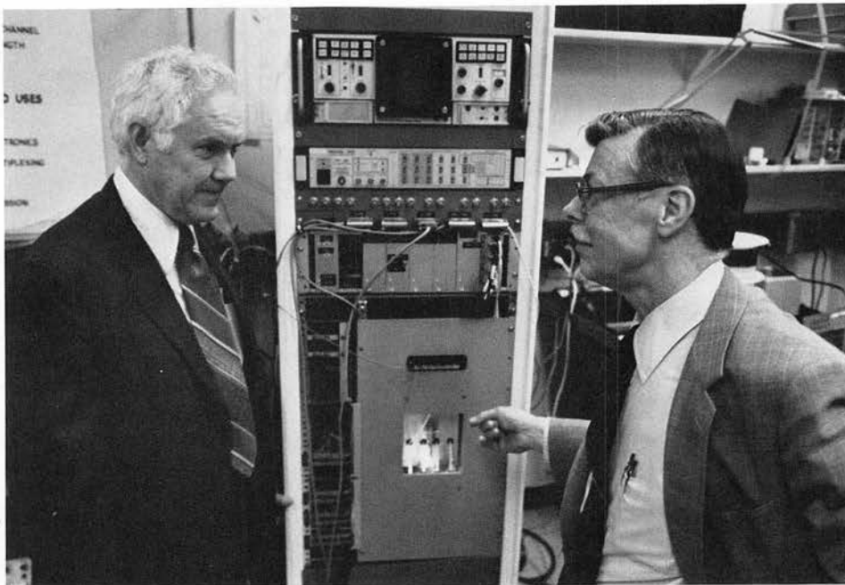
Jim McCrory (right) discusses an experimental lightguide switch with John Stallknecht.
