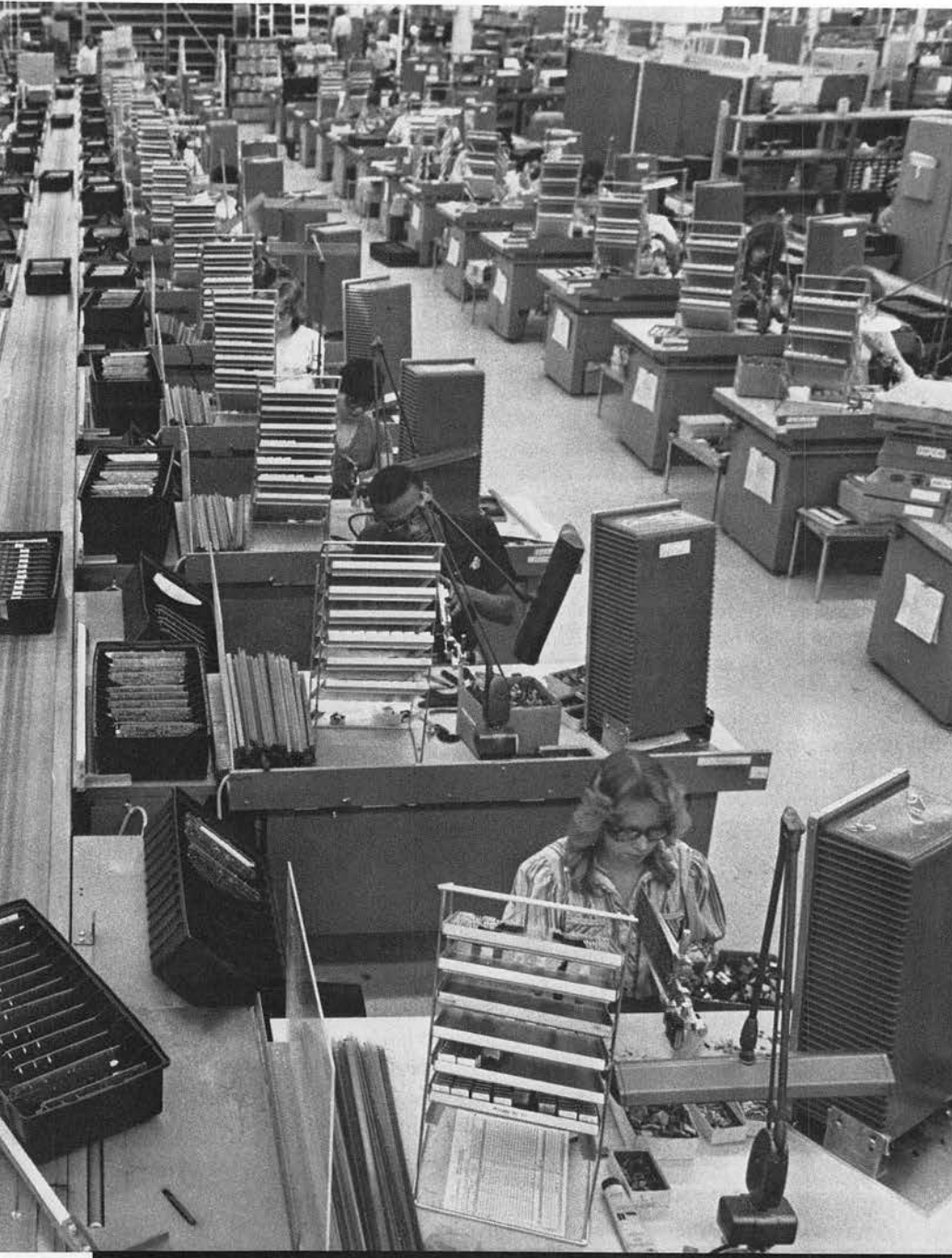
An overview of the transporter, distinctive feature in the assembly of circuit boards at North Carolina Works, where about 1,000 people are involved in the manufacture of SLC-96 systems.
