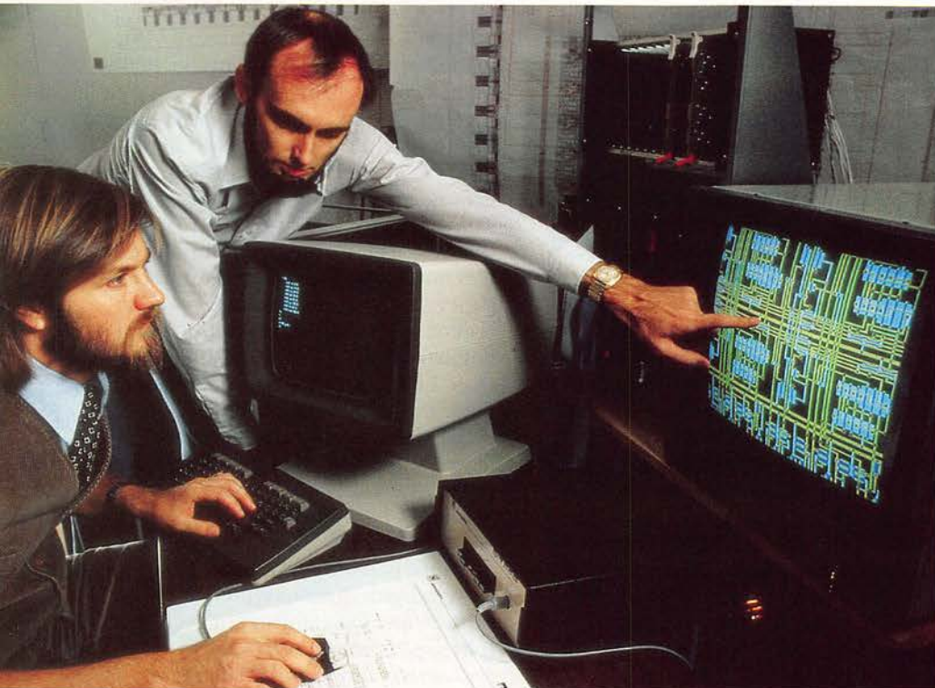
At Holmdel, N.J., Bell Labs engineers use an interactive computer system and a color graphics display terminal to design integrated circuits like the ones in the futuristic photo above.
