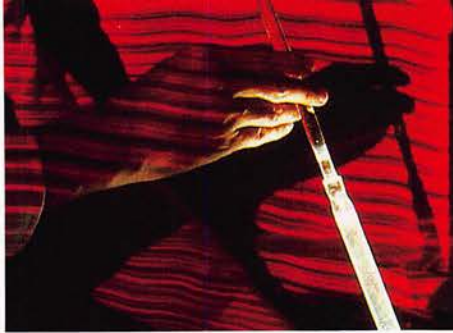
Lightguide fibers are drawn from glass preforms such as this one.
