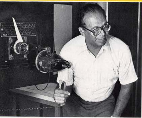
Photographer Bill Debnam shoots 500 to 600 negatives a day on this huge Borrowdale enlarging and reducing camera. The negatives serve as printing plates for most jobs.
