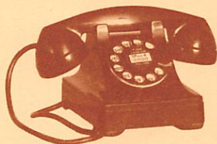
The first desk telephone with the bell in the base.
