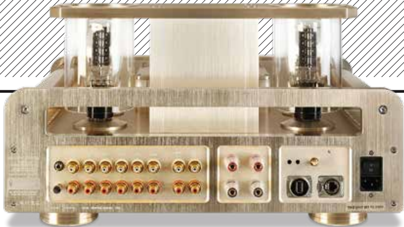
ABOVE: MM/MC phono (with external loading RCAs), four line inputs, line (tape) and preamp outputs are joined by single pairs of 4mm speaker outputs. Antenna services Bluetooth while network (RJ45) and USB-A are for in-factory servicing and updates
